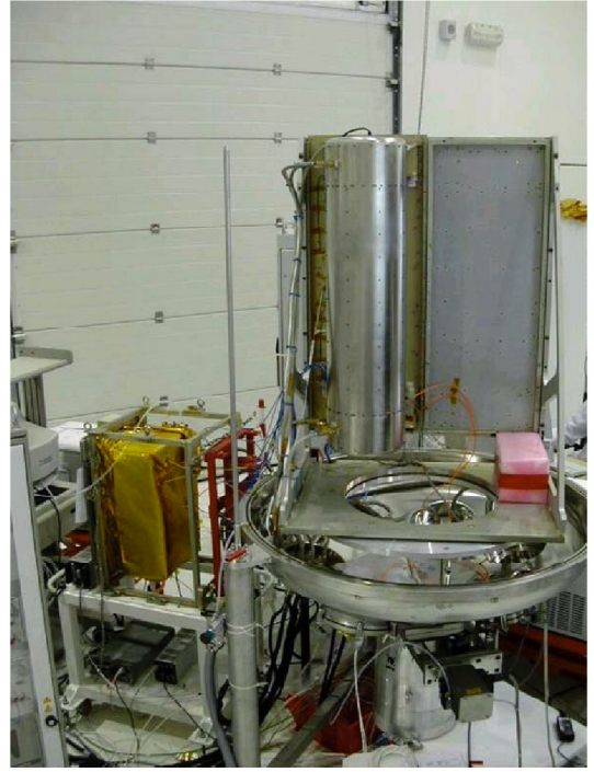
Fig. 7. The PHARAO space clock under test in CNES, Toulouse. On Earth the tube is set vertical. The microwave source is hidden by the tube. The laser source (on the left) is covered with multilayer insulator. On this picture the chamber in which the vacuum tests are performed is opened. The clock can be operated at atmospheric pressure or in vacuum.
